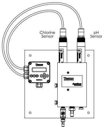
AquaChlor System with free chlorine and pH DataStick sensors installed.
