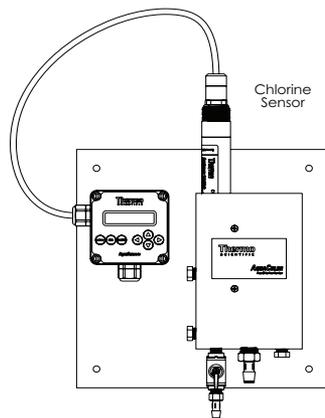
AquaChlor System with free chlorine DataStick sensor only.
