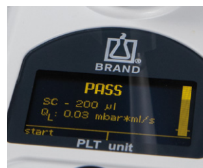
Shows the result and the deviation from the limit within seconds
