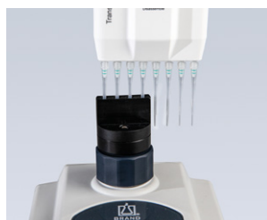
Leak test with multi-channel pipettes
